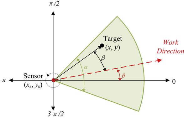
Fig. 5. Illustration for directional model.
