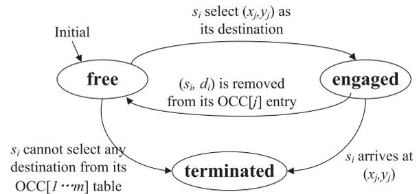
Fig. 19. The state transition diagram of each sensor  $s_i$  in the competition based dispatch scheme [52].
