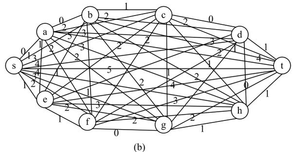
Fig. 11. Sensor network and its corresponding fault tolerant weighted barrier graph when only stationary nodes have location errors. (a) Deployed sensor network. (b) Fault tolerant weighted barrier graph [93].
