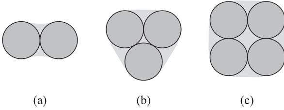
Fig. 8. Illustration of the space points covered by using the  $P$ -probability coverage model of: (a) 2 sensors; (b) 3 sensors; (c) 4 sensors [63].
