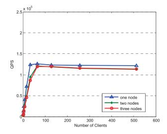
Fig. 6. System throughput of the original Redis cluster.
