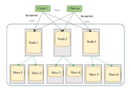
Fig. 1. Overview of a typical client-server structure for Redis distributed storage service.
