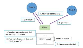
Fig. 4. A use case for client-side key-to-node caching.
