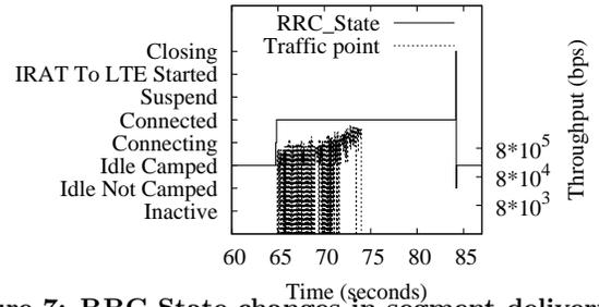
Figure 7: RRC State changes in segment delivery.
