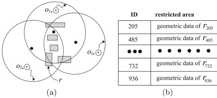
**Fig. 8** Illustrations of the “overlapped” restricted areas and the data structure used to manage the <key,value> pairs. (a) In this example the three candidate moving objects have the same candidate restricted areas. (b) All these data are stored in memory in order to avoid to retrieve redundant data from the database
