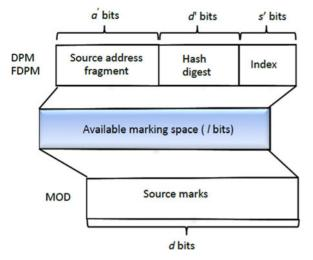
Fig. 3. The comparison between the proposed marking on demand scheme with the typical DPM schemes.
