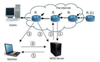
Fig. 2. The framework of the marking on demand scheme for DDoS attack traceback.
