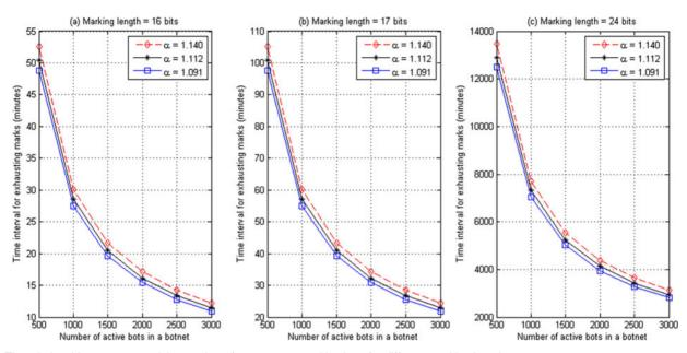
Fig. 6. The relationship among  $T_I$  and the number of concurrent attacking bots for different marking length.
