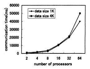
Fig. 3. Experiment about communication contention on CP-PACS Pilot3 ( $P_0$  is the receiving node;  $P_i$  ( $1 \le i < 64$ ) are the sending nodes).
