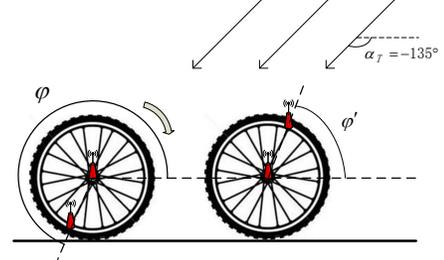
Figure 2: SAR with Two Antennas
