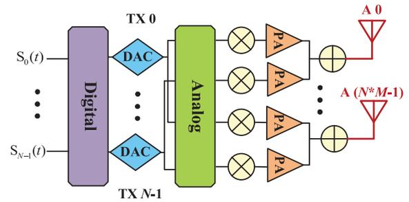
Fig. 3. The structure of hybrid analog/digital beamforming technology for mmWave communications.
