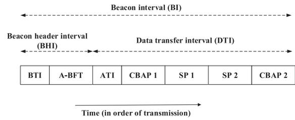
Fig. 14. Example of beacon interval format.
