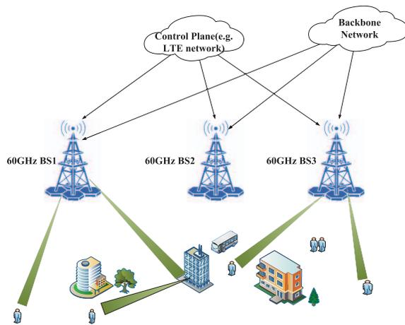
Fig. 4. A potential 60GHz picocell architecture.
