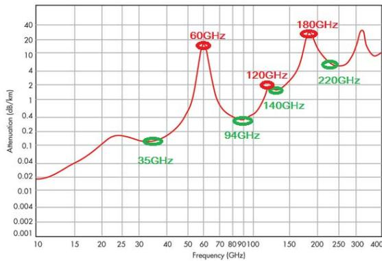
Fig. 1. Atmospheric and molecular absorption at mmWave frequencies [9], [10].
