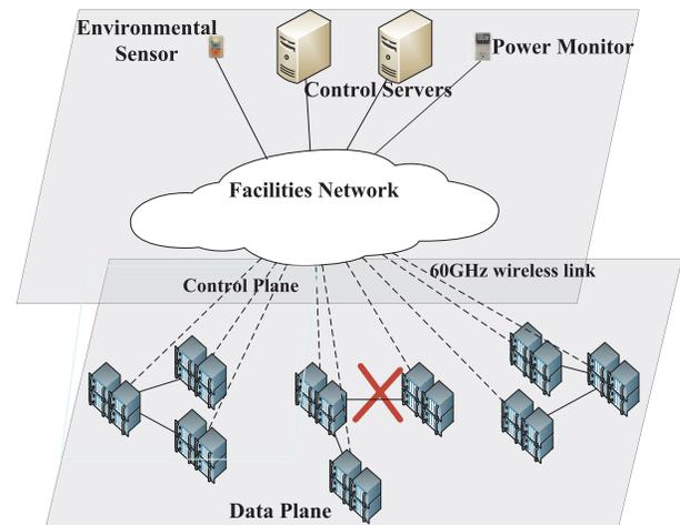
Fig. 5. A facilities network providing robust delivery of control traffic in a data center.
