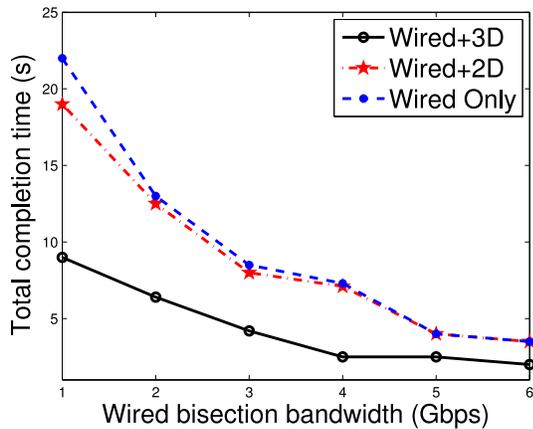
Fig. 9. Overall impact of adding beamforming links.
