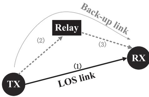
Fig. 6. mmWave relay deployment.
