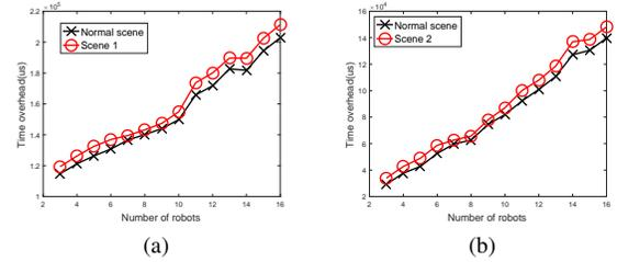
Fig. 8. The time overhead caused by retransmission
