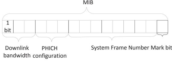
Fig. 3. The structure of MIB in broadcast information
