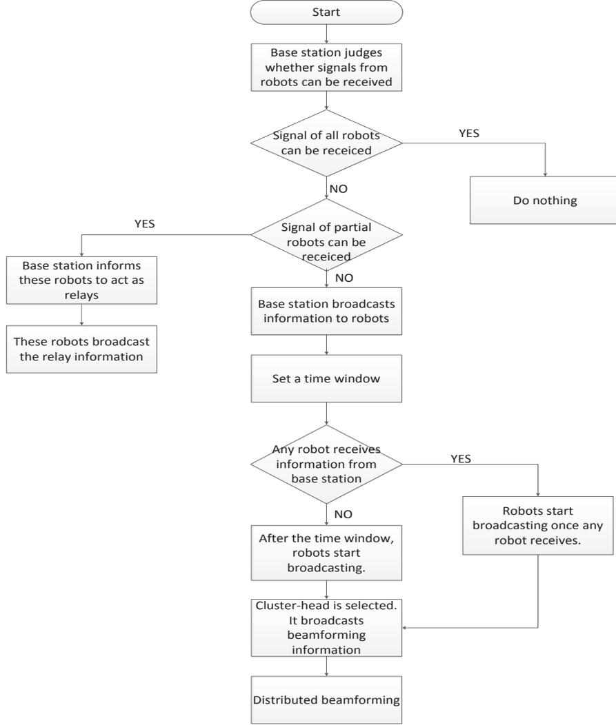
Fig. 2. Co<sup>2</sup>-Robot flowchart
