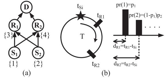
Fig. 7. Illustration examples: (a) A data collection example in low-duty-cycle networks; (b) Computation of expected delay.
