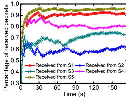
Fig. 1. Packet reception under collisions: the percentage of received packets from each sender.
