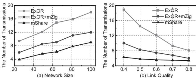
Fig. 17. The performance comparison under different (a) network sizes and (b) link qualities in opportunistic routing.
