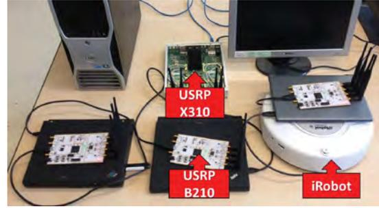
Fig. 8. USRP testbed.
