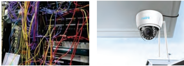
(a) Inflexible deployment of wired surveillance deployment. (b) Easy deployment of wireless surveillance cameras.
