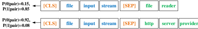
Fig. 3. An illustration of the BERT-based Deep Semantic Ranking Scheme. We pack the keyword sequences of the given method (in blue) and each candidate code sample (in green) into a single sequence separately.
