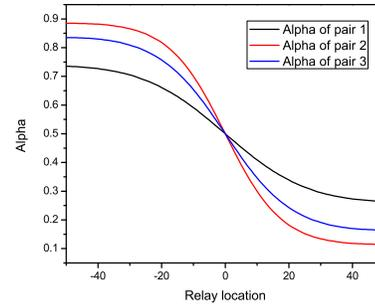
Fig. 3. Alpha vs. relay location (X-axis)
