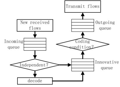
Fig. 3. The control flow at an intermediate forwarder
