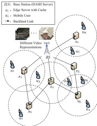
**Figure 1: Example of the system layout, where mobile users are randomly distributed, while edge servers are connected to the base station with backhaul links and can be deterministically placed in the coverage region.**
