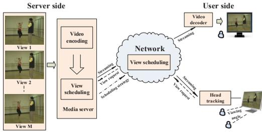
**Fig. 1.** Architecture of interactive MVV streaming system
